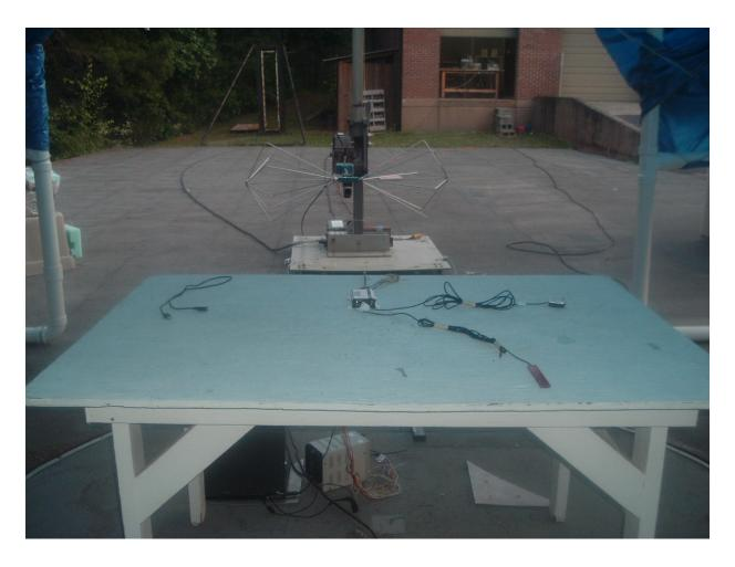
Figure 4 Radiated Emissions (Rear View) from 30-200 MHz
