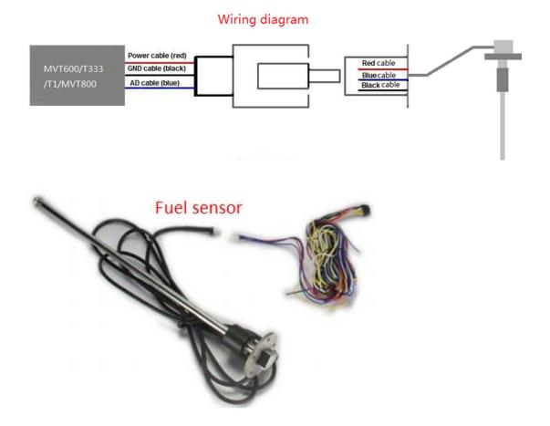
Note: The fuel detection port is a dedicated fuel level sensor port. When a fuel level sensor is connected to the port, no formula is required on MS03. If not, a formula is required.
