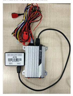
Connect the A78 to two cameras, two A82 seven-segment digital displays and a magnetic card reader:
