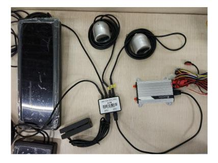
Connect the A78 to the wireless temperature sensor:
